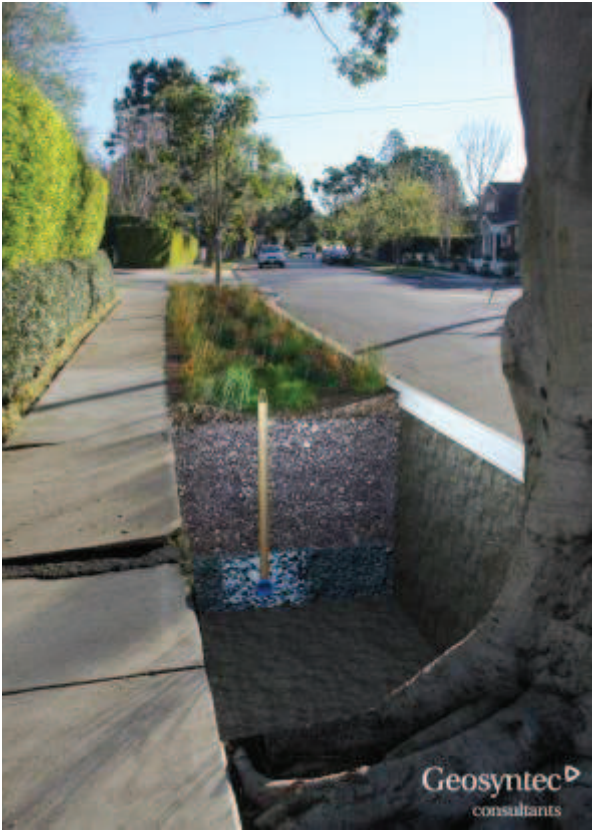
Figure 4-22 Section View of Bioretention with Underdrain
