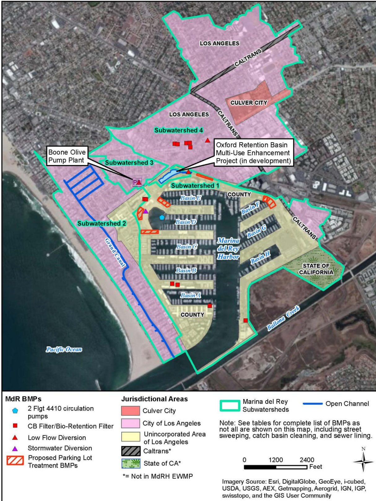
Figure 12. Existing Structural Control Measures within MdrH Boundaries
