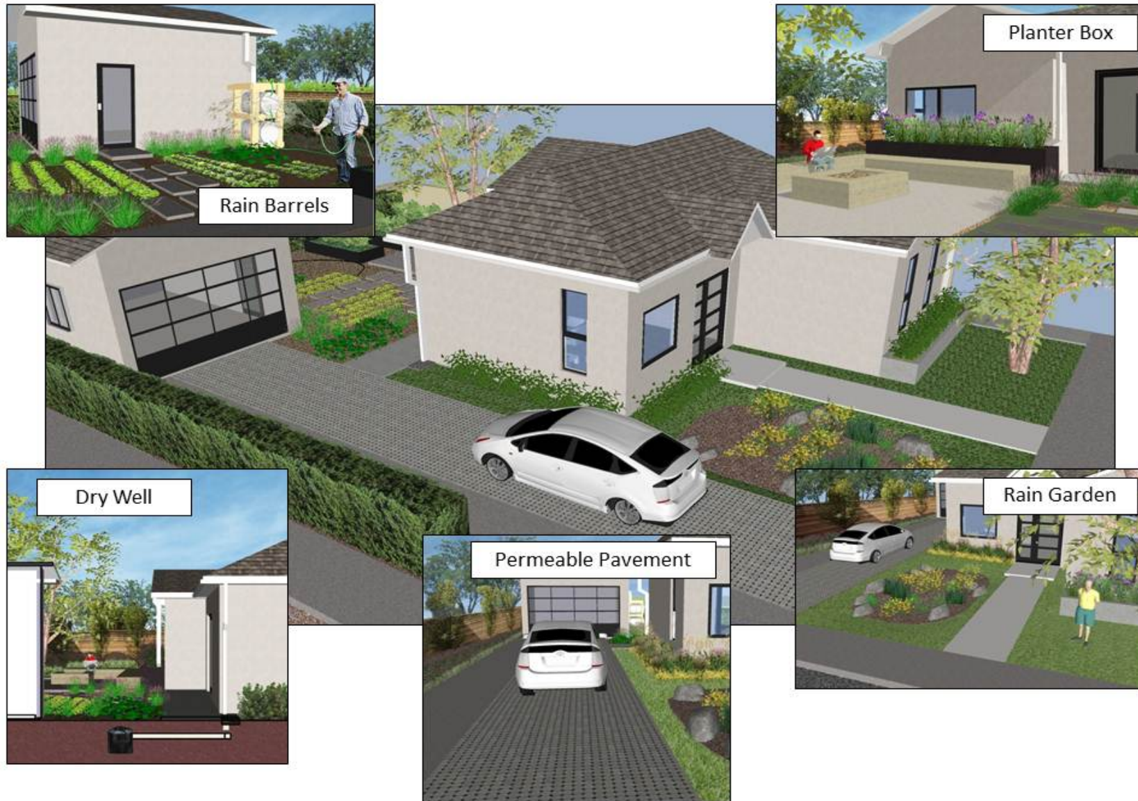
Figure 3.1- Small Scale Residential BMP Schematic
