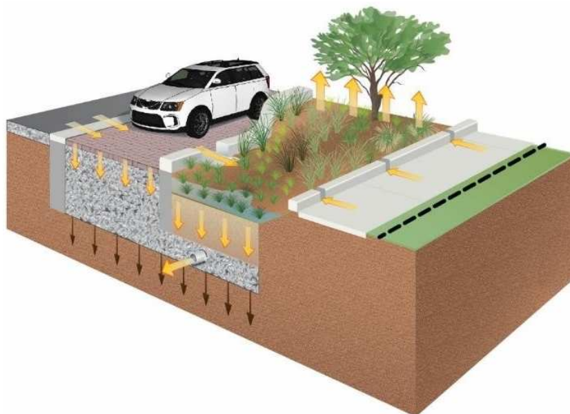
Figure ES-3 Conceptual Schematic of a Green Street (arrows indicate water pathways)
